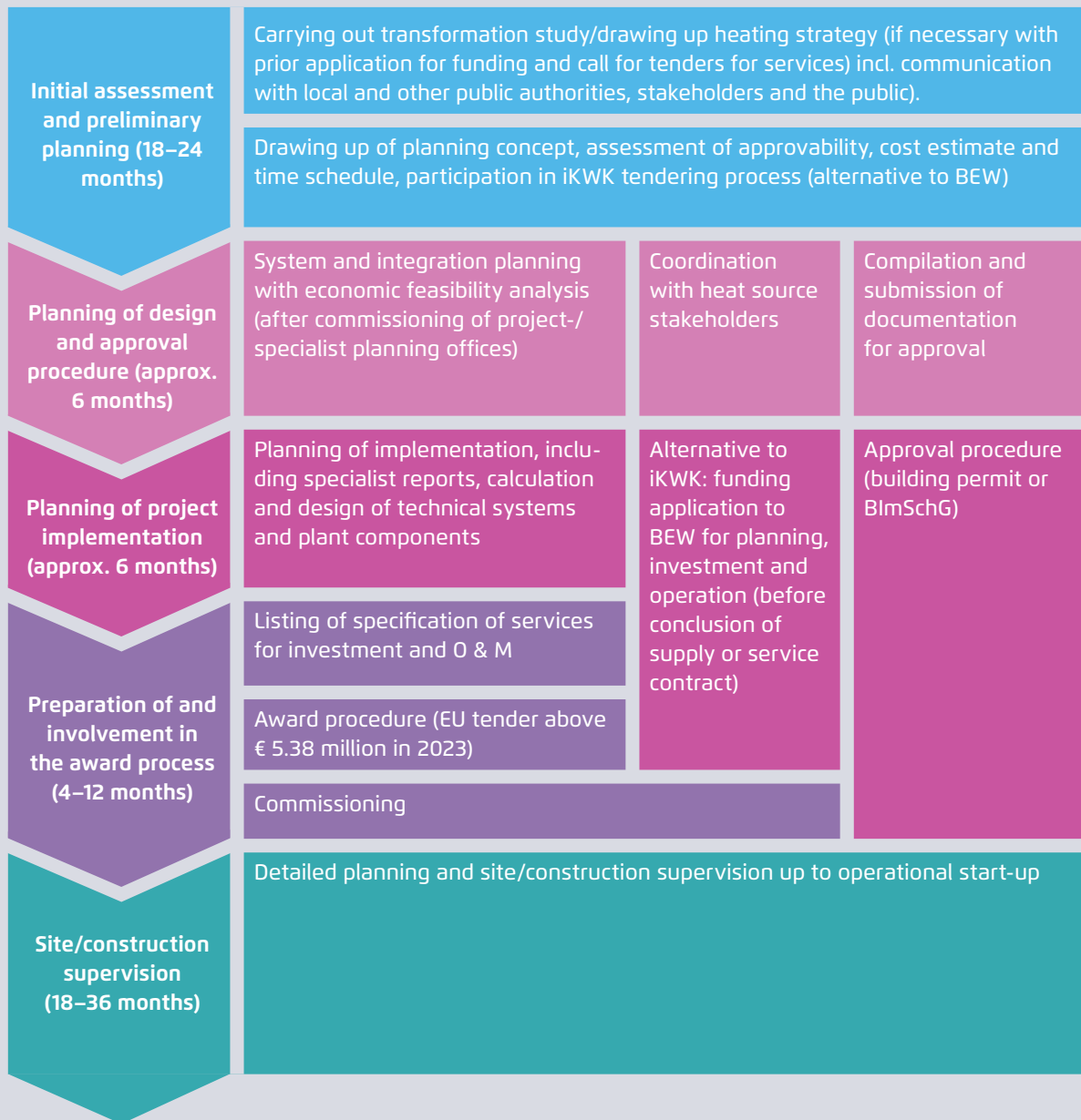
Phases of a large-scale heat pump project showing the most important tasks with approximate duration in months
